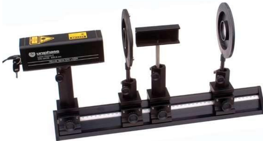
Fig. 4: Experiment setup “Classical Interference Experiment”. Position of components (left edge of the optical rider): laser: 0 mm, lens f = 5 mm: 150 mm, Fresnel mirror: 220 mm, lens f = 200 mm (only mounted when the distance to the virtual light source is measured): approx. 380 mm. The interference image is obtained on the screen (or a brightly lit wall) at a distance of 2 to 3 m.
