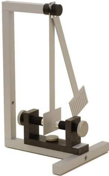
Fig. 5: Experiment set up for “induced eddy currents”
